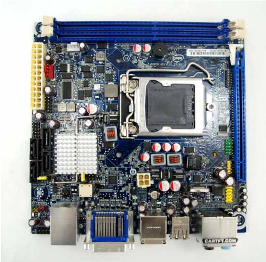
As mentioned in the specification you can find some more usefull connectors onboard. So you can find for example six USB (3 via Pinheader), four SATA (RAID functionality), one eSata and one PCIe port.
