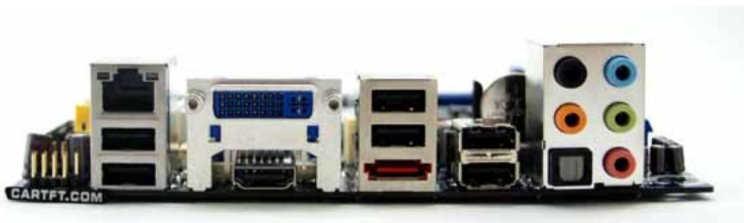
The backside of the new Mainboard looks very good. Additional to the standard I/O ports you can find a DVI, one HDMI, one eSATA and one SPDIF Connector which can realize a lot of different usages.
